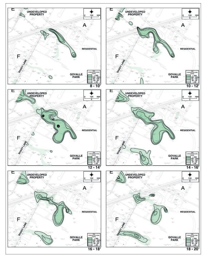
**FIGURE 11.** TPH screening analyses "slice" maps, showing the areal extent of TPH concentrations at various depth intervals (slices) over the interval 8 ft to 20 ft (2.4 m to 3 m) below the ground surface.
