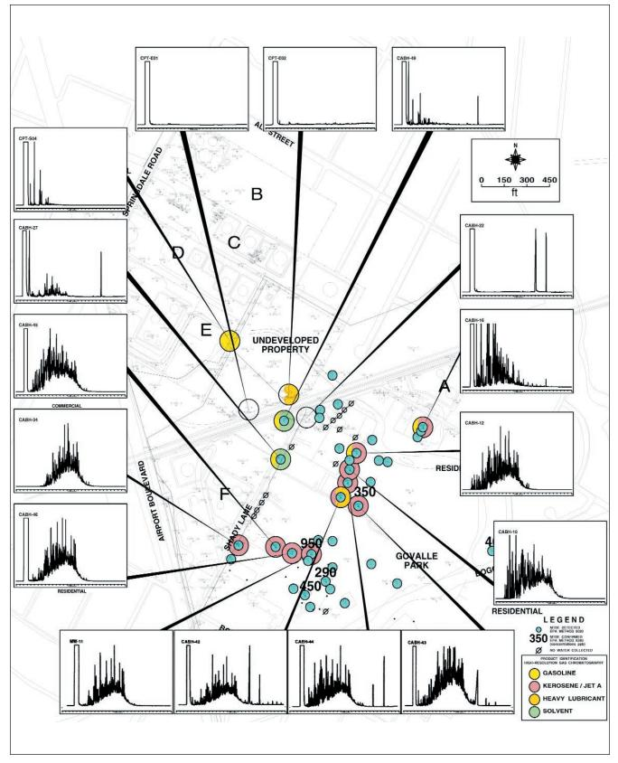
**FIGURE 18.** Map of study area, showing product types identified in fluid (NAPL and groundwater) samples collected from borings and monitoring wells using high-resolution capillary gas chromatography. Product types are color-coded in accordance with the legend at lower right. High-resolution capillary GC chromatogram signatures are shown for each boring and monitoring-well sample analyzed.
