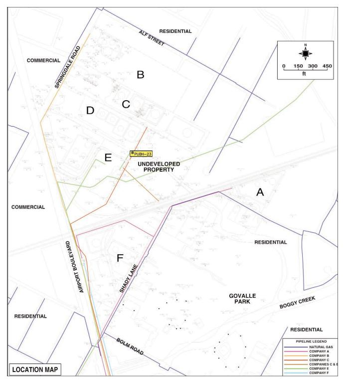
**FIGURE 1.** Location map of study area, showing the six former bulk storage and distribution terminals and pipeline properties (A-F) and surrounding city of Austin park (Govalle Park) and residential and commercial properties. The locations of pipelines, boreholes, and monitoring wells are also shown.
