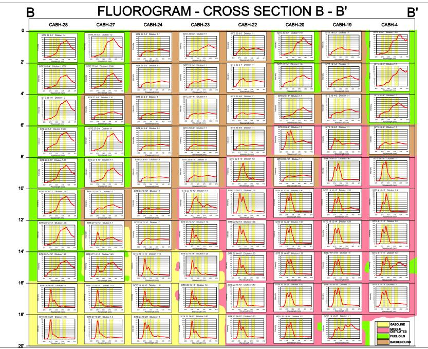
**FIGURE 7**. Cross-section B-B' showing fluorograms for each 2 ft (0.6 m) soil core sample collected and analyzed in various borings. Note variations in intensity and contaminant type in individual borings and along the line of section. Different product types are color-coded in accordance with the legend at the lower right.
