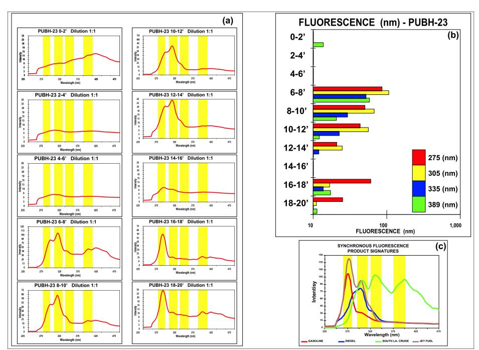
**FIGURE 6**. (a) Fluorograms showing product types identified in soils from the ground surface to -20 ft (6 m) in boring PUBH-23. (b) Bar graph showing the fluorescence data for various wavelength windows (in nm). (c) Standard fluorescence signatures for gasoline, diesel, crude oil, and jet fuel.
